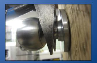
1 - The Maxximus Rexx, by necessity as a prying tool, doesn't have the ramp that the Rex Tool does. Therefore, it doesn't grab rim and mortise cylinders as aggressively (though that was not a problem in any of our tests).
