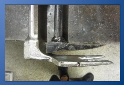
5 - The Maxximus Rexx, despite having no aggressive ramp, did a fantastic job of biting through or around collars and onto rim and mortise lock cylinders. Second only to the standard Rex Tool, we would say.
