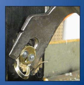
6 - The greatest <u>disadvantage</u> of the Maxximus Rexx as a lock-puller lay in the shape of the adz. Because the lock-pulling jaws are slightly off-set to the shaft, it has a tendency to turn to the right and can be difficult to steer back to a neutral position.
