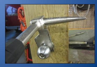
4 - With the bifurcated adz of the Maxximus Rexx, it's easy to drive one tooth of the adz behind the collar of most key-in-knob and deadbolt locks. Not unlike using a Mini Pro Bar or Truckman's Tool.
