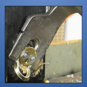
7 - Another disadvantage of the Maxximus Rexx is that it is somewhat awkward to use by <u>yourself</u> as a lock-puller, as it was a bit cumbersome to hold the tool with one hand (though that's how it was used in nearly all our lock-pulling tests).
